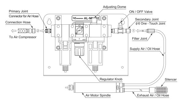
Fig. 16 Connection of Air Line Kit " AL - M1202 (Sold Separately) "
