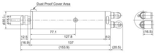
\* 90°Angle type airjoint is free to rotate for the direction of Air flow.
