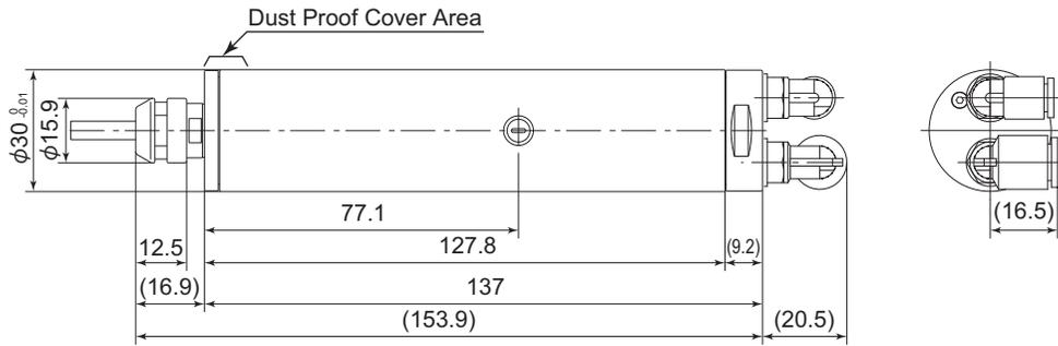
\* 90° Angle type airjoint is free to rotate for the direction of Air flow.
